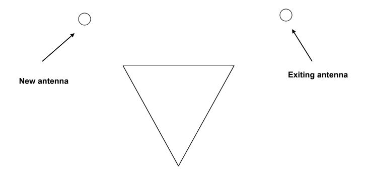
Mounting the antenna off a tower leg is the best way to go. Since the antenna is producing a strong field at every azimuth angle, getting the antenna further away from the tower usually produces the best results. If possible aim for more than 2 Lambda from the tower (at 600 MHz 39 inches or 100 cm).
