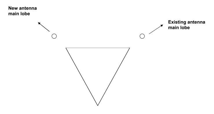
If the Omnioid antenna is going to be mounted on the face of the tower, try to mount it as far as possible away from the tower. A good rule of thumb is a minimum of 1-3/8 Lambda. At 600 MHz that would work out to 27 inches (69 cm).
