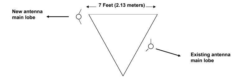
When mounted as depicted by the drawing above, the two antennas will cause minimal pattern disruption to each other. Electrical isolation between the two antennas is between 30 dB and up to more than 50 dB depending on the difference in frequency of operation.
